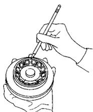
Figure 2. Checking the rotor web area.
