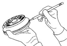
Figure 3. Checking the outer rim of the rotor.
