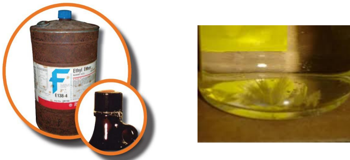
Figure 2. Examples of chemical containers showing signs of crystal formation
