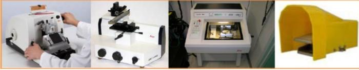
(L to R) Rotary, Sliding and Freezing (Cryostat) microtome and foot treadle guard
