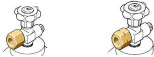
The conventional right hand threads for non-flammable, non-toxic gases.
