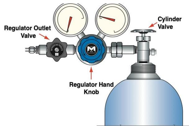
Figure 1. Components of gas cylinder and regulator assembly
