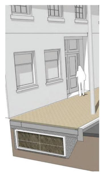
Type 2: On-grade pavement over soil cells
