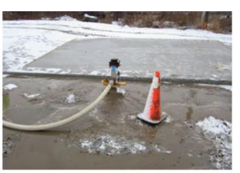
Water introduced - water bursting out of saturated soil adjacent to installation.
